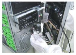
3. Release the ODD rails and disassemble the two ODDs.
